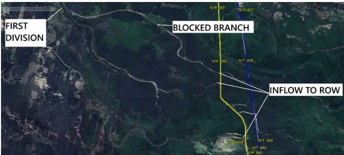
FIGURE 6: POINTS OF WATER INFLOW INTO THE ROW
