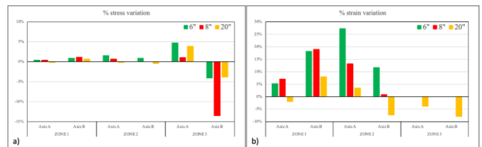
FIGURE 20: EVALUATION OF % CHANGE PACKAGE 2 a) STRESS VARIATION. b) STRAIN VARIATION.
