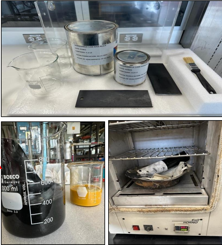
Preparation of the low friction coating RBCF - (Sigmashield 1200)
