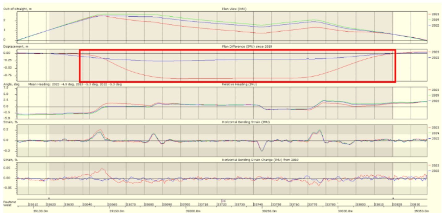
FIGURE 12: DISPLACEMENT IS EVIDENT IN THE PLAN DIFFERENCE PANEL.
