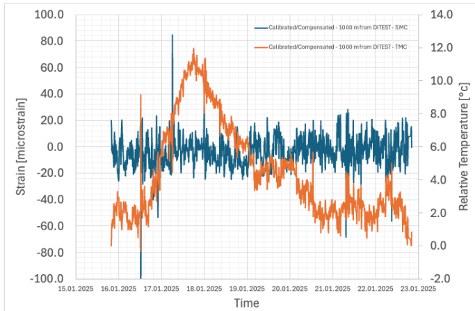
FIGURE 18: CALIBRATED AND THERMALLY COMPENSATED MEASUREMENTS (STRAIN IN BLUE AND TEMPERATURE IN ORANGE) FOR SENSOR 3 O’CLOCK AT 1000M FROM THE INTERROGATOR.
