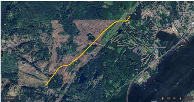
FIGURE 5: PIPELINE ROUTE (ORANGE LINE) THROUGH THE BLUE LAKE (CRESCENT LAKE) AND RED BLUFFS LANDSLIDES.
