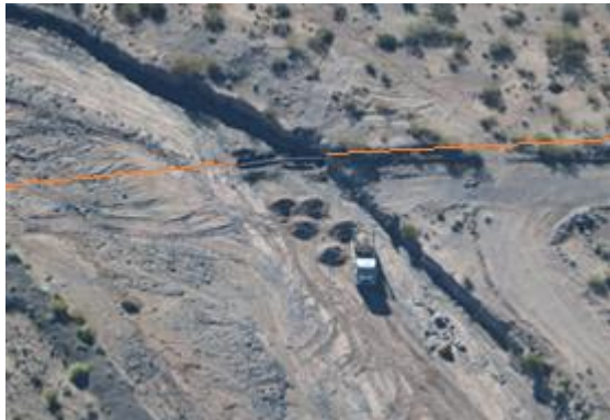
Image 5 – Aerial view of exposed pipeline – Source: Aereal patrol
