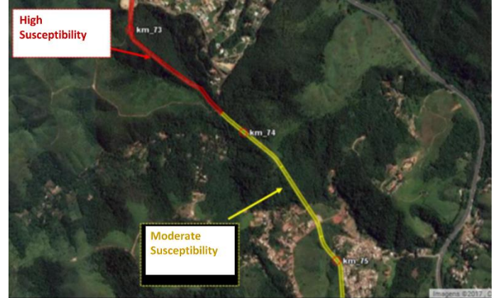
FIGURE 8: AERIAL PHOTOGRAPHY REVEALING COMPOSITE SUSCEPTIBILITY ZONES (HIGH, MODERATE, AND LOW) FOR MULTIPLE RISK TYPES.
