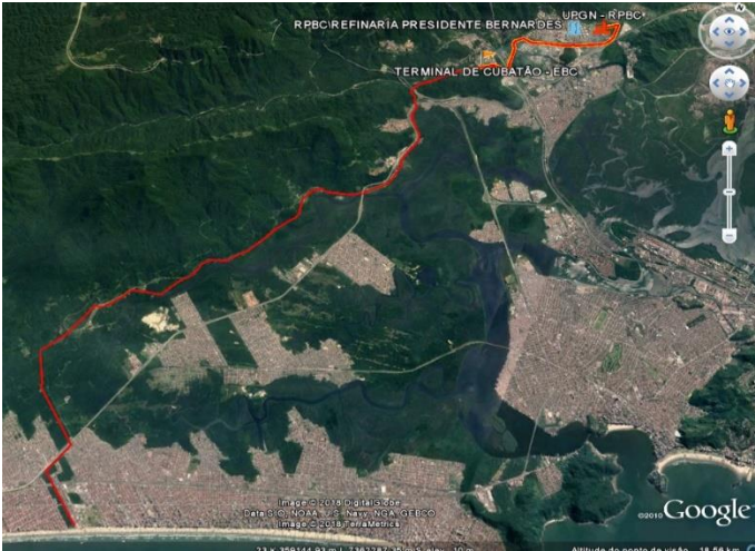
FIGURE 1: PATH OF THE 16" GAS PIPELINE, EXTENDING FROM THE SEAFLOOR (SUBMERGED ALONG THE COASTLINE) TO THE REFINERY, NAVIGATING THROUGH DIVERSE TERRAINS, INCLUDING MULTIPLE MARINE SOIL DEPOSITS.
