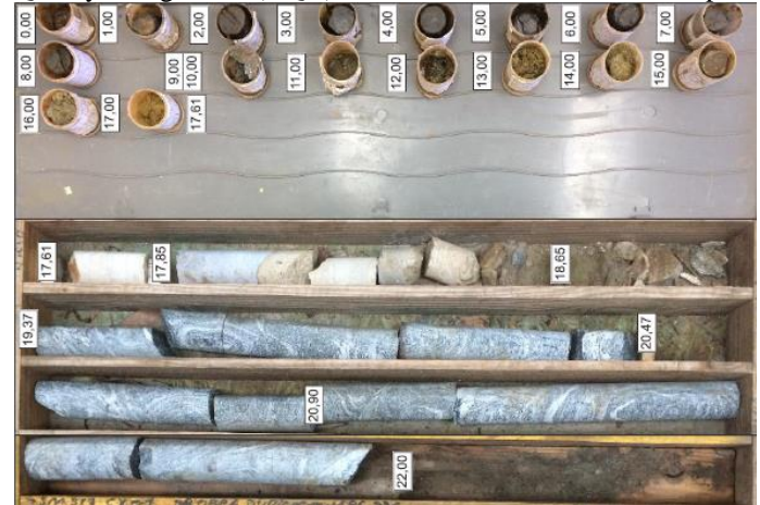
FIGURE 17: ROCK SAMPLES IN THE RQD TEST.
