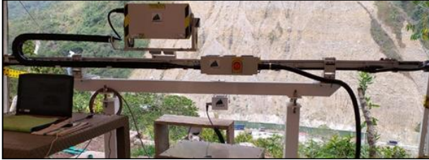
FIGURE 2: LISA TYPE GEORADAR FOR 24/7 REMOTE MONITORING OF THE K58-MESA GRANDE
