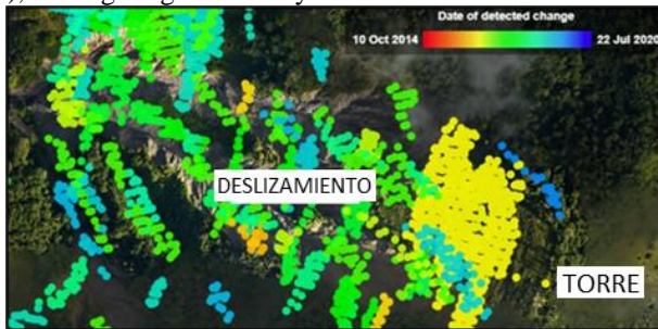
FIGURE 12: HISTORY OF EVENTS DUE TO AMPLITUDE CHANGES IN SATELLITE SIGNAL AROUND A POWER TOWER
