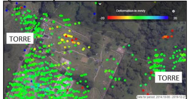
FIGURE 10: DEFORMATION RATES IN THE ANALYSIS AREA FOR THE PERIOD 08/10/2014 – 27/12/2019
