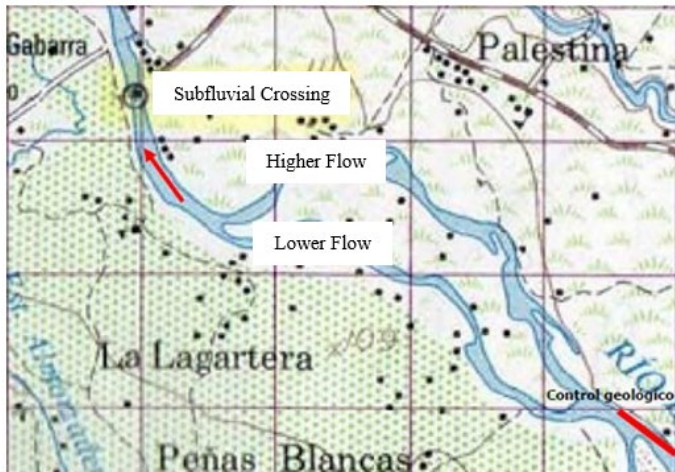
Figure 8: Configuration of the Blanco River with two branches before the sub fluvial crossing.
