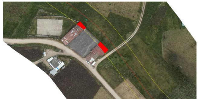
FIGURE 6: IDENTIFICATION OF ROW ENCROACHMENT DETECTED WITH UAV. Source: OcenSA.
