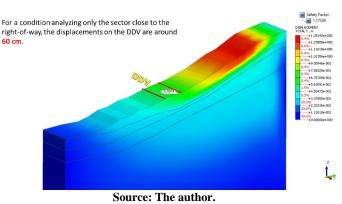
A longitudinal model was also carried out to determine the thrust forces of the calculated displacements, as well as those that would be supported by the semicircular casing of alternative 1B.
