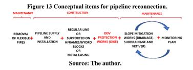
In maintenance, work must be done together and based on the results of the monitoring plan in order to update, improve or repair the corresponding mitigation works.
